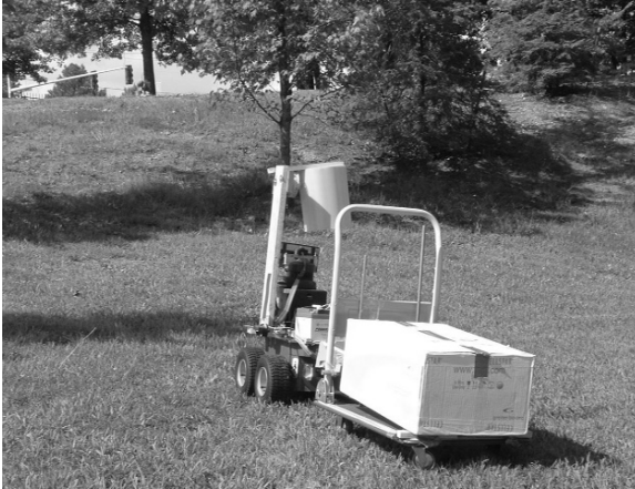
Fig. 9.2. Pioneer AT robot pulling a loaded cart up a hill.
